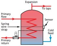
The gravity tapstat may be fitted in the primary flow line if preferred
